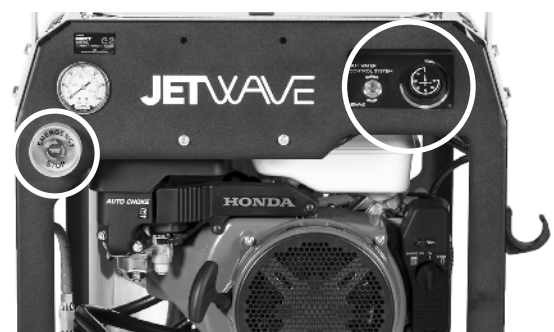
Figure.8 - Explorer G2 E-Stop & Burner Operation
