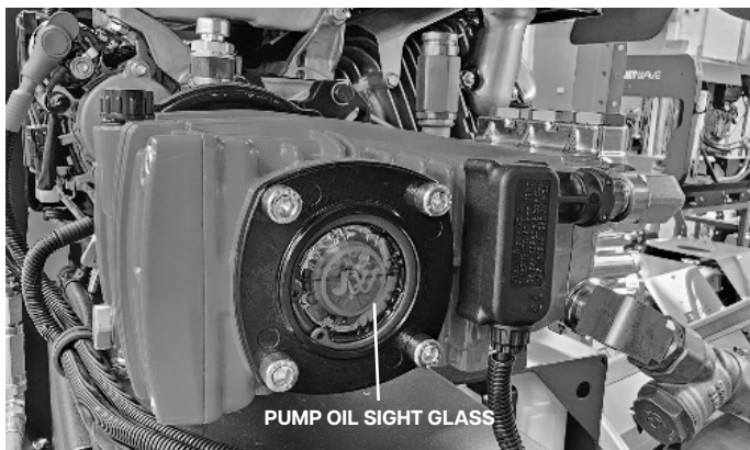
Figure.10 - Checking Pump and Gearbox Oil Level
