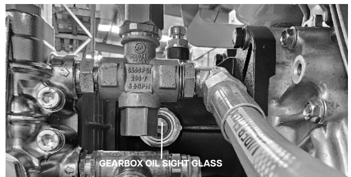
Figure.11 - Checking Pump and Gearbox Oil Level
